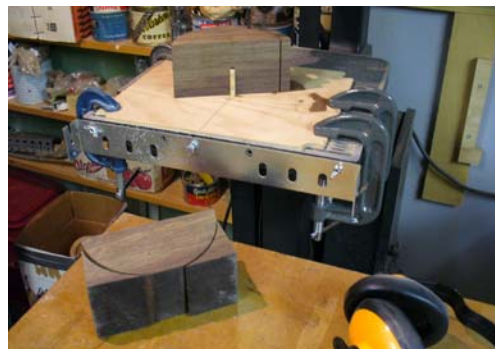
First vertical cut into 1st half block. Band saw set-up in background, pivot pegs fastened into block halves
