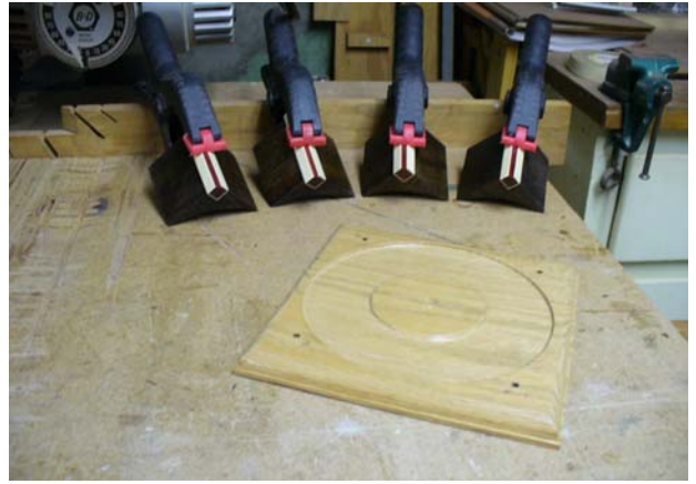
Gluing of stand's corner strips to block corners are seen in upper part of photo
